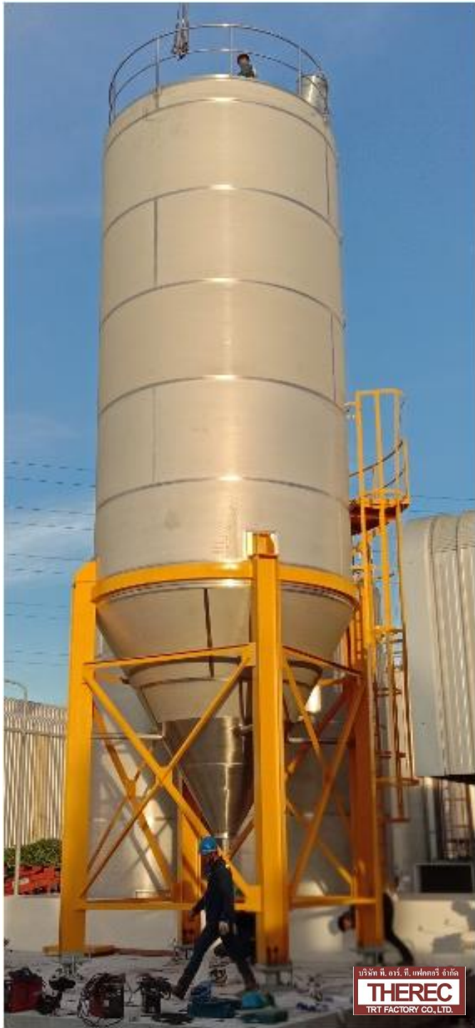
Stainless steel 304 PVC Resin Silo, Size 100 m 3
