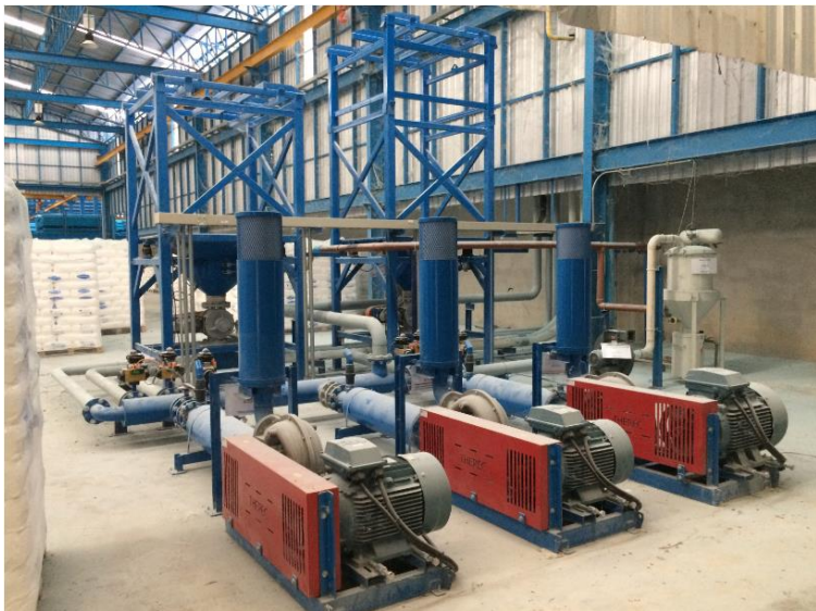
PVC & CaCO 3 Bulk Bag , Silo feeding system, 5 Tons / hr
