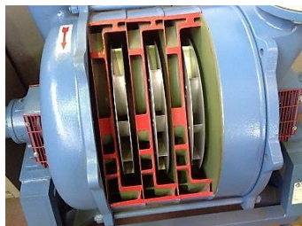
Internal Parts / Impeller / Drum (housing) / Static part
