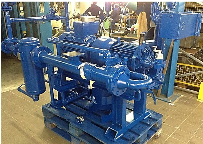
First “Mapro” Rotary vane Gas Compressor In Thailand for Palm Oil Bio-gas Plant
