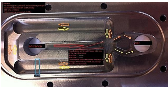
Oscillating Principle of Measurement
