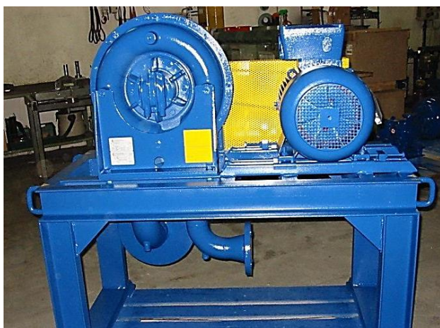
Belt Drive Upside Down Blower Package to avoid the water trap
