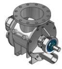
Out board bearing blow through, powder & pellet handling rotary valve for high vacuum & pressure pneumatic conveying system
