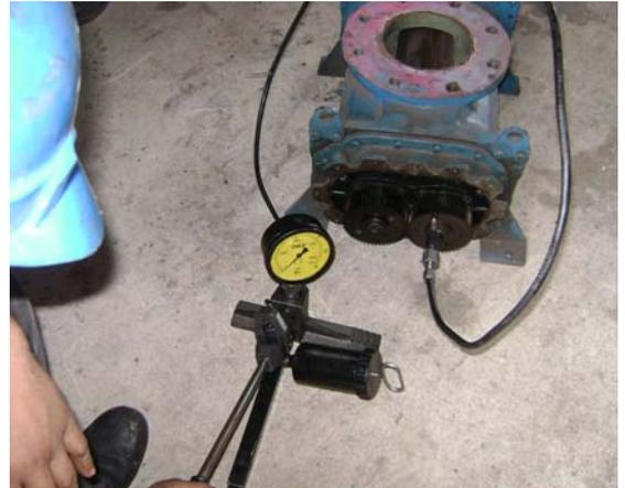
Super High pressure hydraulic hand pump "SKF",
