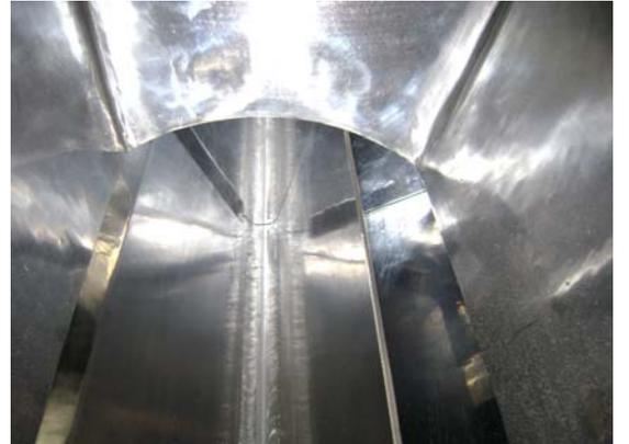
SIZE 6.0" ,SUS 304, with water cooling chamber ,for car coolant film scrap recycle, pneumatic conveying system
