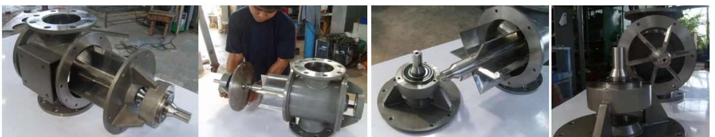
Easy Detachable (Quick Cleaning) Valve, Garlic Powder, SUS 304, Size 150 mm
